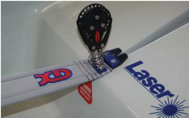
3 Fit new **XD hiking strap** and **ratchet block** using the spring and shackle provided.
