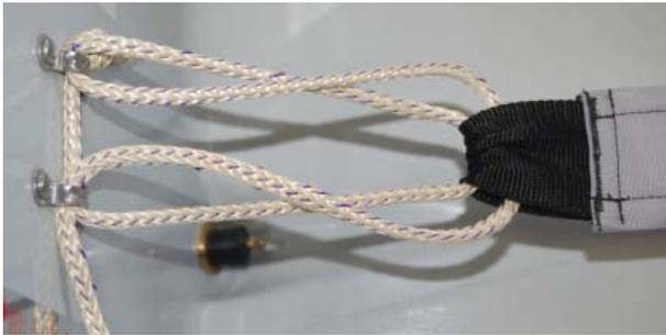
**9** The rope tail is then passed through the starboard eye so that the end of the V12 can be pulled from the side of the boat.
