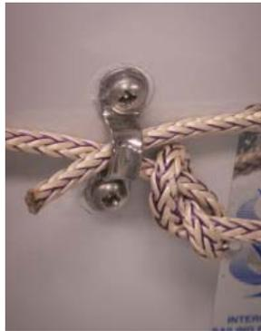
7 Next pass the tail around the port eye feeding it from the outboard port side.
