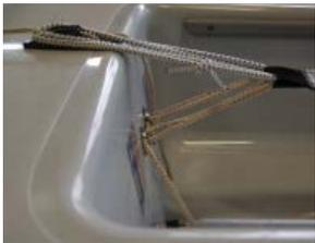
**11** Tie the mega bungee to the hiking strap by wrapping it around the traveler cleat and hiking strap twice before tying the ends with a reef knot. The bungee will be tight.
