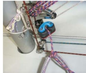
**14** Feed the control line through the plastic **tube** supplied and tie a bowline to form a handle, which is also a stop knot that you can set up to your desired maximum ease setting. Make sure the knot on the block and becket is just short of the top block.
