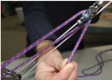
**10** Continue to feed the Dyneema control line back through the bottom block from the starboard side top block in the body of the base unit.
