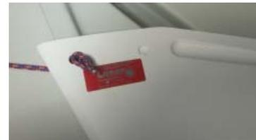
**15** Put the free end tip through the daggerboard hole when sailing for ease of access.
