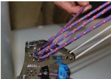
**11** Continue to feed the Dyneema control line back up to the double block, feeding the line from front to back.
