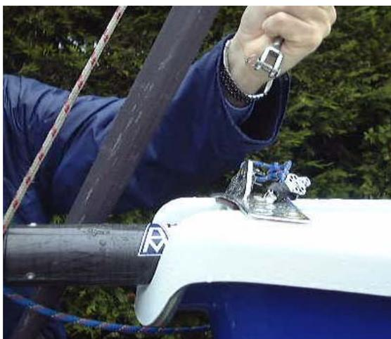
19. Using the winch **SLOWLEY** wind the rig forward to engage the forestay clevis pin. Attach the ring to the pin and then release the winch. **DO NOT OVERWIND THE WINCH.**
