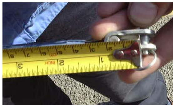
7. Fit the V2 / D4 ( Caps)shrouds and the V1 / D3 ( main shrouds) to the T terminals first and then to the spreaders. The Ferrules on the main shrouds are located as shown. Locate the Main shrouds into the spreader end by removing the clevis pin and slotting into position. The clevis pin then fits to the bottle screw on the Cap shroud.
