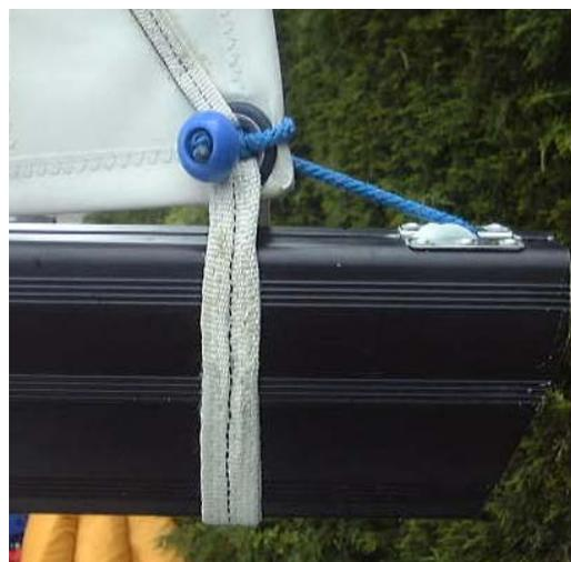
7. Hoist the sail with the bow sitting head to wind. **The sails should be stowed for launching and recovery of the boat.** Care should be taken when hoisting the sail and should always be fed into the sail feeder to avoid jamming and tearing the sail. Attention especially to the top batten protector.
