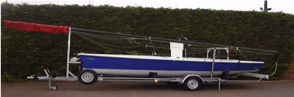
3. The mast and cradle are moved aft. The mast cradle should be positioned at the back of the boat as shown, and then the mast is moved aft to position the mast heel to the step.
