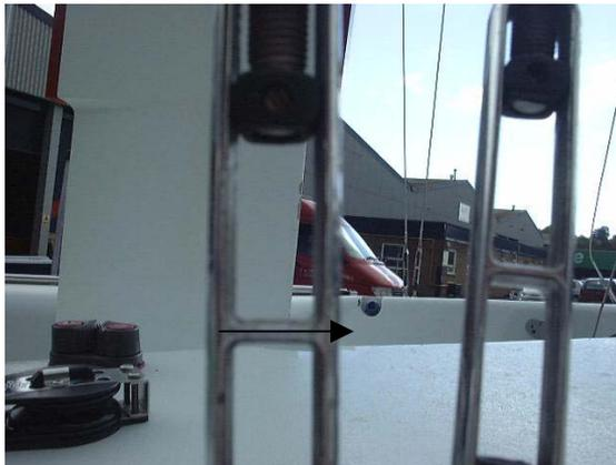
Lock the shrouds by using a small screwdriver and rotating the grub screw anticlockwise to secure bottle screw.
