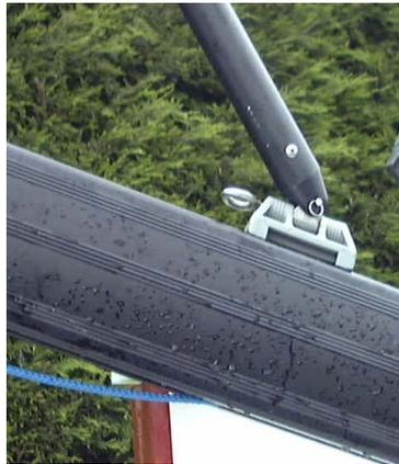
4. The Gnav tackle ( supplied with Gnav bar ) should be attached by taking the only free end of the black / green fleck rope and feeding this thru the sheave on the top of the boom.
