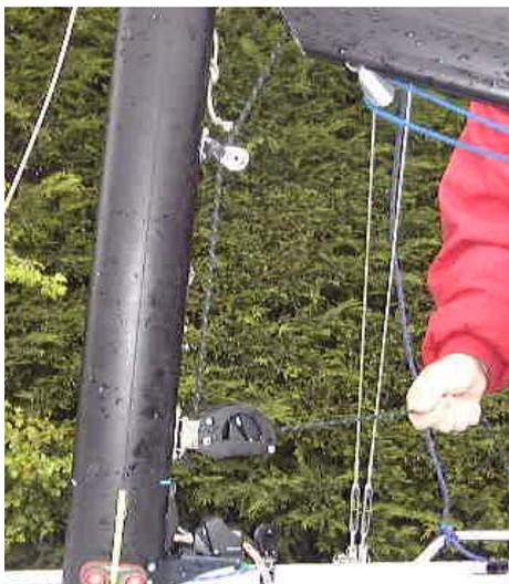
6. Attach the pulley and shackle on the black / green rope to the lower D ring / webbing on the mast.
