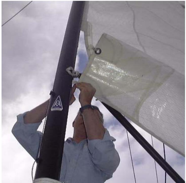
8. When the sail is fully hoisted the two plastic slides should be fed into the cut out in the mast luff groove just below the Gnav bracket. The outhaul should be eased at this point to assist this operation.
