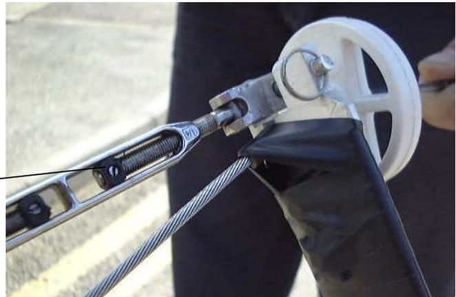
10. V1 / D3 shrouds - Adjust the bottle screws so that they are the same length and showing approx 20mm of thread. (loose, this will be set up once the rig is raised and tensioned)
