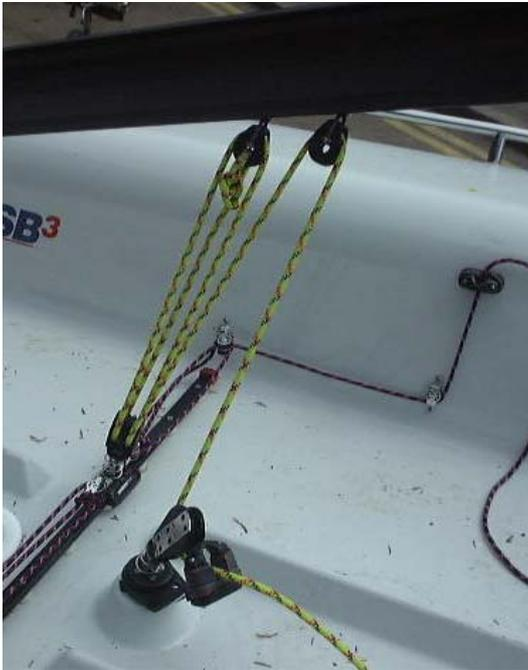
1. The mainsheet is dead-ended at the rear block on the boom by tying a bowline thru the block.
