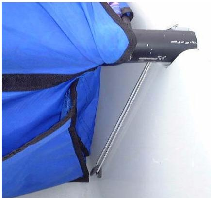
4. Insert the starboard end and secure the elastic to the clip
