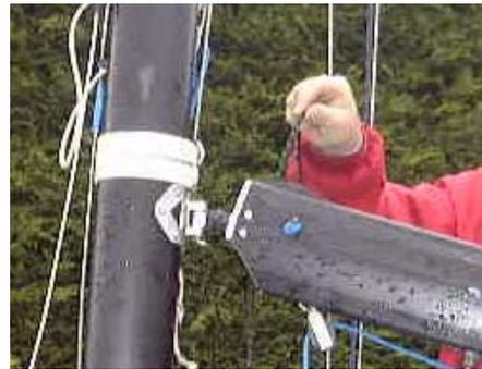
5. Feed this rope thru the pulley on the aft face of the mast and then to the top spinlock cleat.
