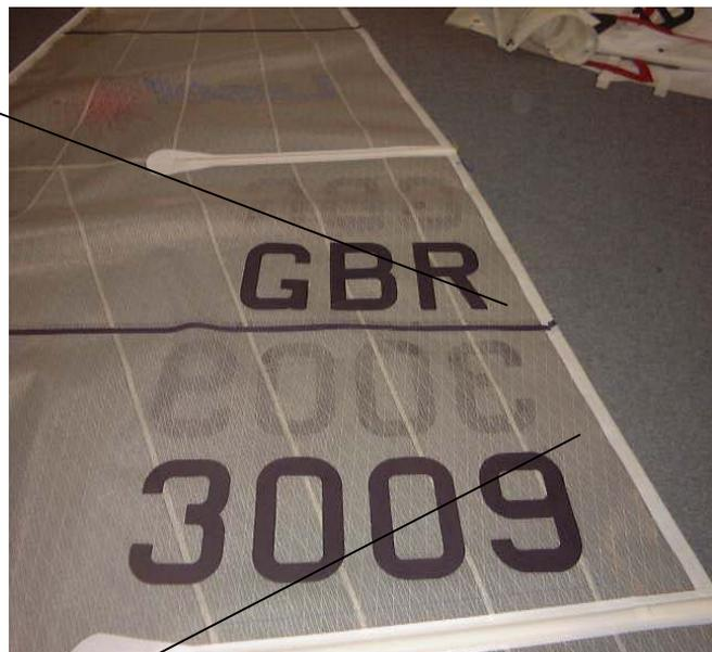
12. The starboard side GBR should be positioned 60mm above the port side letters and parallel to them.
