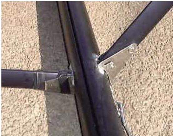
5. The spreader is fixed with no adjustment. They are marked port and starboard and simply attached with two clevis pins and rings. Ensure that these are taped up.
