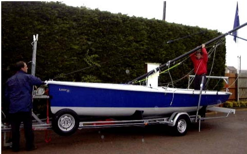
18. With the mast in the upright position – take the gennaker halyard and secure it to the trailer. Cleat off the gennaker halyard at the mast. This is purely as a safety line whilst attaching the forestay.
