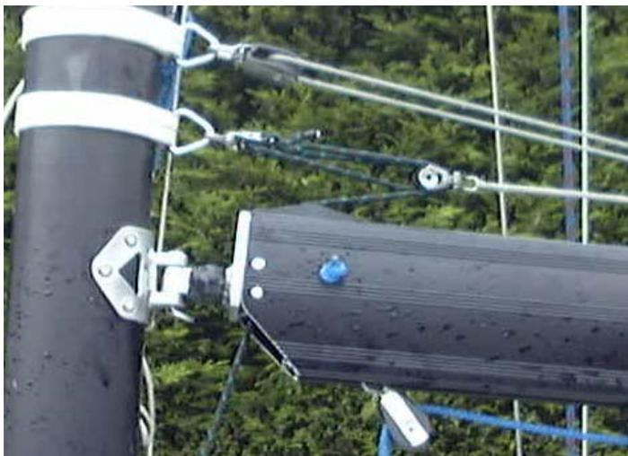
8. Attach the last pulley and shackle to the uppermost D ring and webbing on the mast
