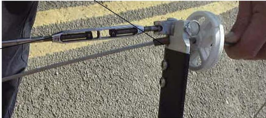
8. Tape up the main shroud as shown. This holds the feral in position whilst fully taping the end of the spreader assembly.
