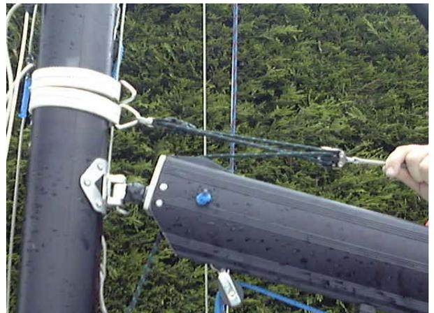
7. Attach the large pulley and shackle to the Gnav car on the boom.
